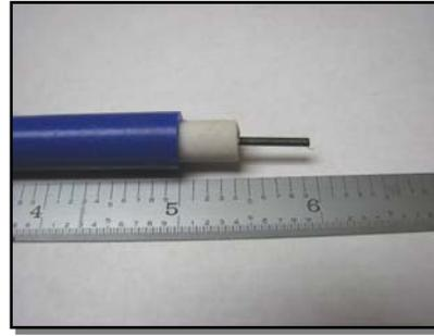
After you have measured and cut the wire(s) to the correct length, strip back  $\frac{1}{2}$ " of white insulation surrounding the center core, *without damaging the core!* Next, cut and strip  $\frac{3}{8}$ " of colored outer jacket without cutting into the white inner insulation. Next, carefully fold over the center core. Insert the wire into the terminal with the core next to the bottom of the terminal and form the terminal tabs around the wire to hold it in place for crimping.
