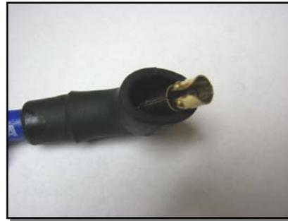
For the early style socket type terminal, put a slight bend in the terminal to aid in the boot installation. Insert the terminal/wire into the boot. Carefully bend the terminal up into a 90 degree configuration to fit the boot correctly. (You do not have to bend the terminal when using the late model HEI style boot/terminals).
