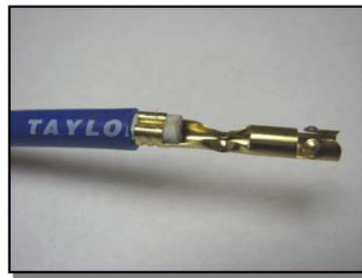
Slide a piece of heat shrink tubing over the crimped connection and apply heat with a heat gun or hair dryer. Be careful not to catch the heat shrink tubing on fire, as it will burn with excessive heat.
