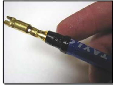
Put some of the silicone grease on the terminal and heat shrink tubing. Spread it around the terminal to aid the installation into the distributor boot.
