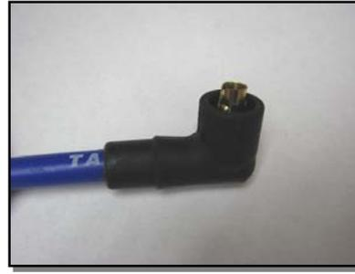
The steps for the HEI style terminals are similar to the conventional terminals except bending the HEI terminal is not required during insertion into the distributor boot.
